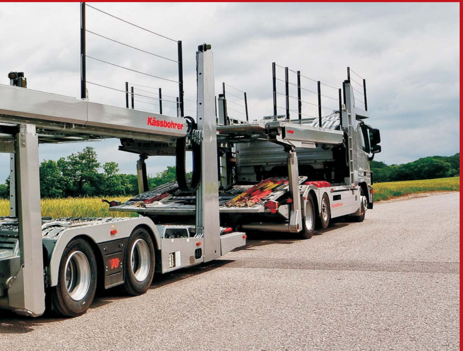
Twin tyred for high load capacity and rolling bellows for exceptional stability.
