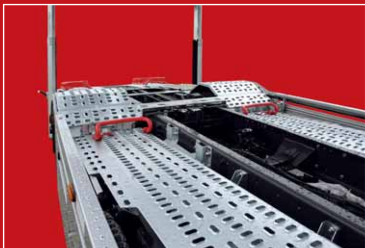
Optimum loading height is assured by hydraulic lowering of the lower platform tracks.
