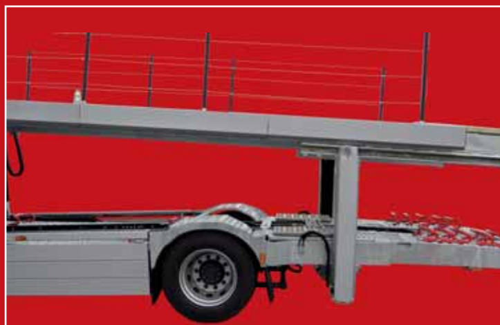
Rear lifting device in high-strength steel alloy for quick loading and unloading.
