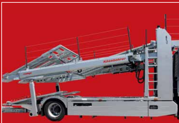
Innovative hydraulic kick-up ramps offering maximum loading flexibility.
