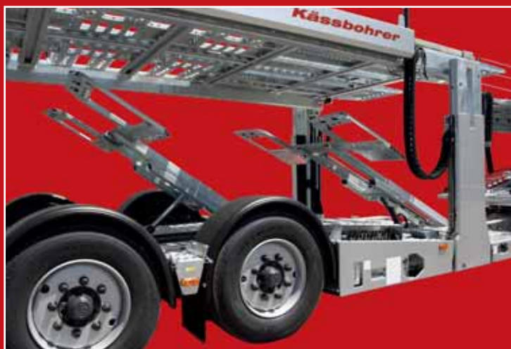
Simple and precise loading with the hydraulic kick-up ramps guarantees safe load positioning.
