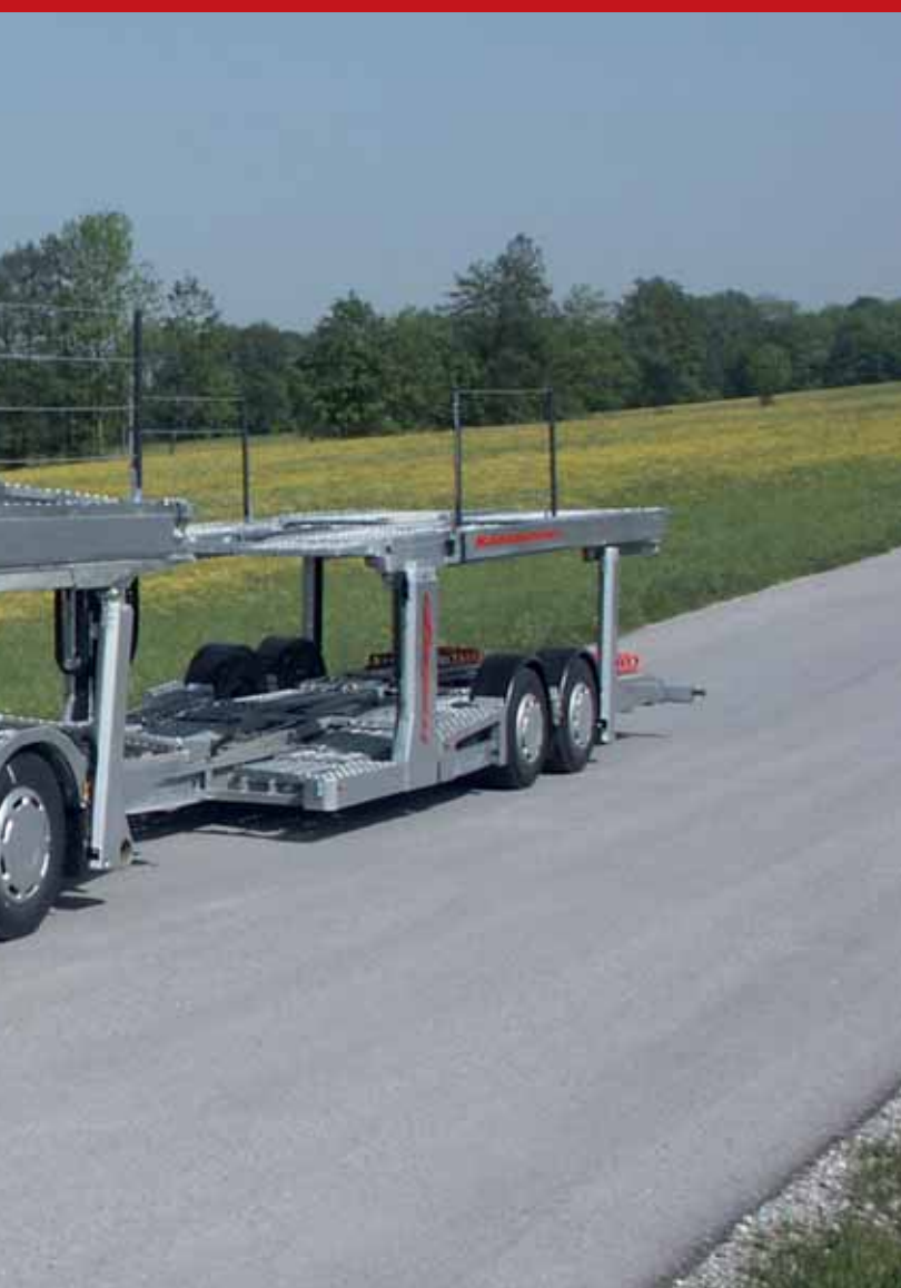
Lifting system at the trailer's front end has been designed to provide maximum loading width at the upper platform.
