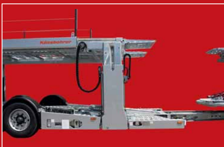
Lifting system at the trailer's front end has been designed to provide maximum loading width at the upper platform.
