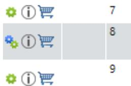
The double gearwheel means that the displayed assembly branches again into a subassembly with individual parts. The
